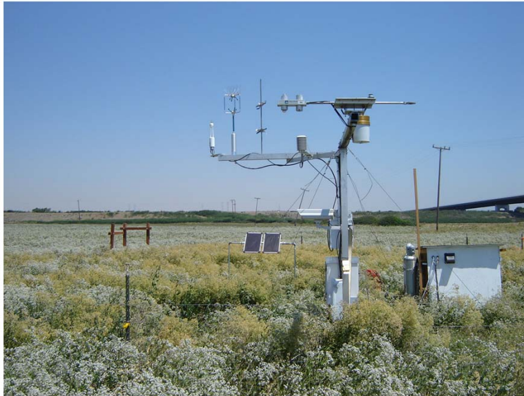
Typical Micrometeorological Flux Instrument Station
