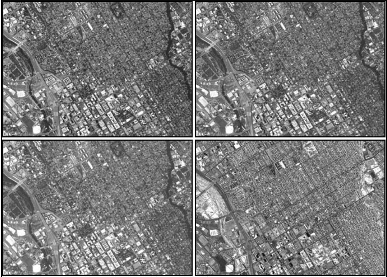
Figure 2. Sample images of each band. Top left: band 1 (red), top right: band 2 (green), bottom left: band 3 (blue), bottom right: band 4 (near-IR).
