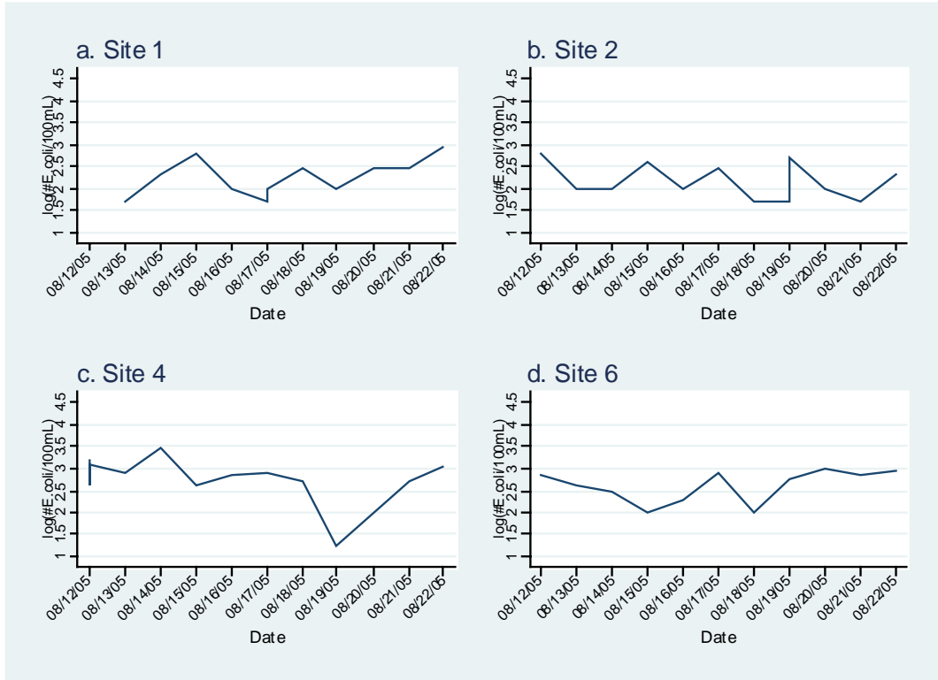
Figure 3.4: Day-to-Day Variability in Water Quality at Four Stream Sampling Sites on Estero Maria over the Course of 12 Days (8/11/05-8/23/05) during the dry season: a) Sampling Site 1; b) Sampling Site 2; c) Sampling Site 4; d) Sampling Site 6. Sites 1, 2, and 4 were sampled between 09:00-12:00 each day and Site 6 was sampled between 14:00-16:00. Upper limit of detection is 4.65 (45,000 CFU/100 mL); Lower limit of detection is 1.70 (50 CFU/100 mL).
