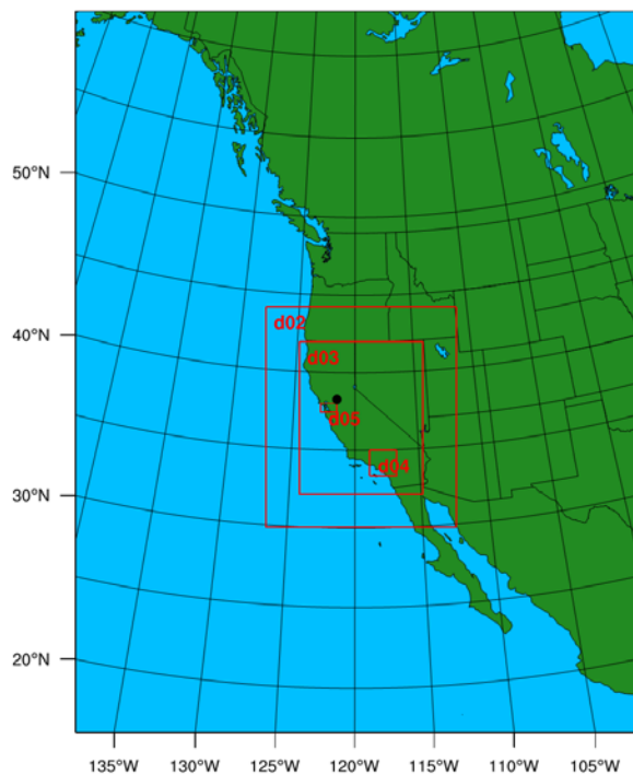
Figure 5.3. WRF initial boundary set up with three-level nested domains. The ratio of spatial resolution between the three levels is 3. The resolutions for d01, d02, d03 and d04/d05 are 36, 12, 4 and 1.3 km, respectively.
