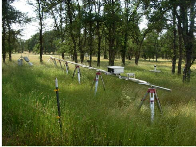
30 m Tram System, with Up and Down PAR and Rnet
