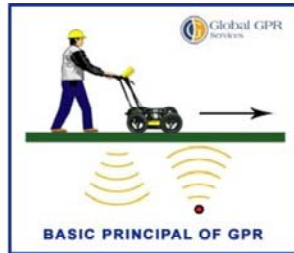
Ground Penetrating Radar
