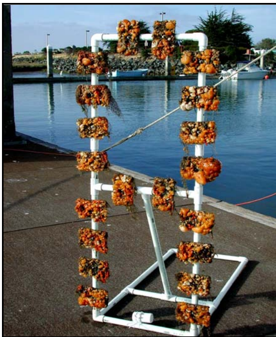
Figure 1: Fouling panels attached to the PVC rack. Each panel is 10cm X 15cm. The rack is normally suspended under the floating dock such that the surfaces of the panel which are visible in this picture face downward.
