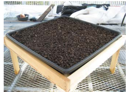
Figure 2. Non-vegetated modular extensive green roof, “soil module”
