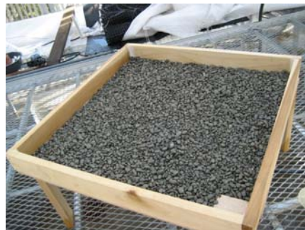
Figure 3. gravel roof model, “gravel model”
