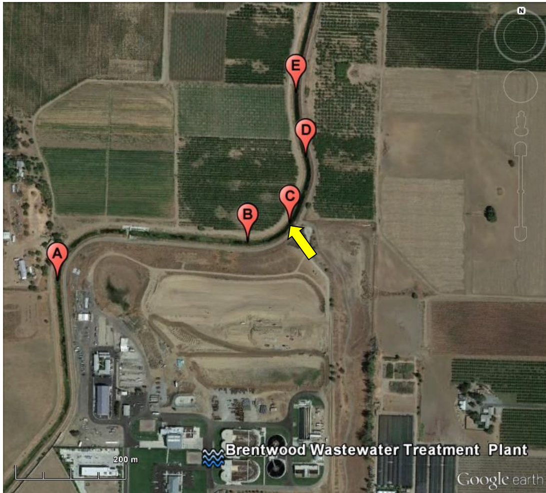
Fig. 1. Aerial map of sample locations and BWTP. The yellow arrow indicates where the recycled water enters Marsh Creek. Sites A and B are located upstream of the recycled water effluent. Sites C, D, and E are located downstream of the recycled water effluent. The constructed drop-structure and fish ladder with an installed USGS stream gage is located between sites A and B.
