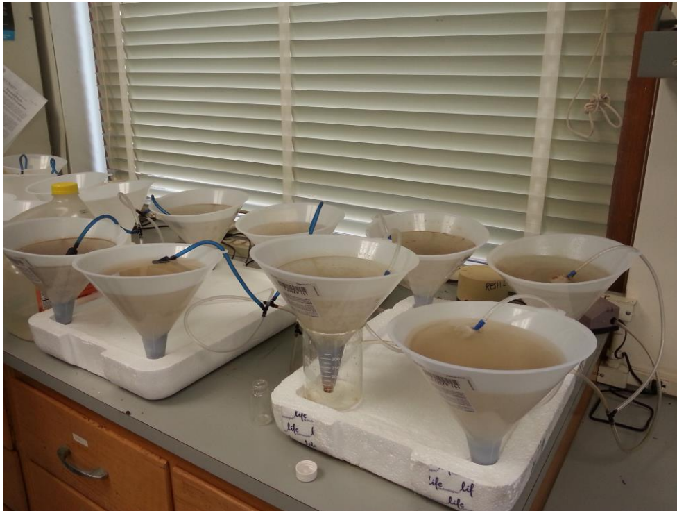
Figure 2. A picture of the experimental design. 16 funnels were spread over five rectangular pieces of Styrofoam.
