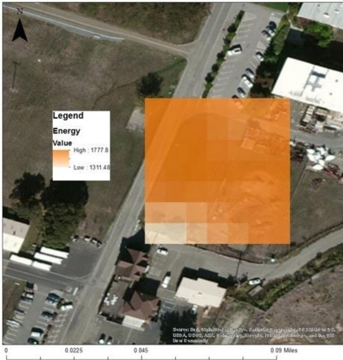
Figure 2. Annual Solar Energy Map. Raster map showing range of solar irradiance levels that the study site receives. Ranges from 1311 to 1778 kWh/m 2 /year
