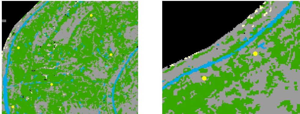
Figure 7. Accuracy Error in NCM: Because the scale parameter of the objects was smaller to capture finer water channel details, validation point classifications created by assessing the original imagery were difficult to match with areas classified as a heterogeneous mix of mudflat and vegetation. The yellow points in these images show pixels that had been classified as vegetation based off Google Earth imagery and the false color display of the original IKONOS imagery, but were classified as mudflat with the nearest neighbor configuration algorithm.
