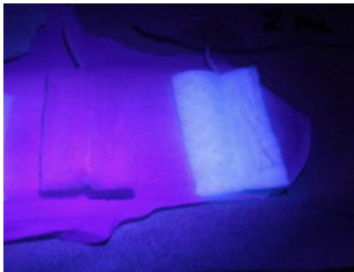
Figure 1. Samplers that were illuminated with a non-branded 375nm-395nm UV handheld light from a local hardware store to detect fluorescence a. Non-Fluorescing cotton-pad sampler (left, entire cotton-pad does not fluoresce) b. Fluorescing cotton pad sampler (right, entire cotton-pad does fluoresce).
