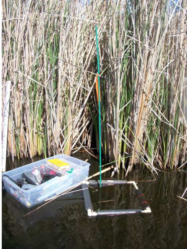
Figure 3.7: Experimental Field Setup for Light/Dark Incubations (Mayberry Farms). PVC frames that delineated sampling regions were kept in place by attachment to stakes. I tied BOD bottles to the PVC samplers and hung them \sim 10 cm below the water surface for the approximately one hour duration of productivity experiments.
