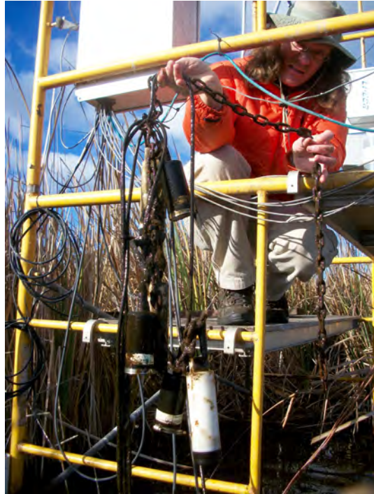
Figure 3.2: Servicing YSI meters for long-term aquatic data collection at Mayberry Farms, atop an eddy covariance tower.
