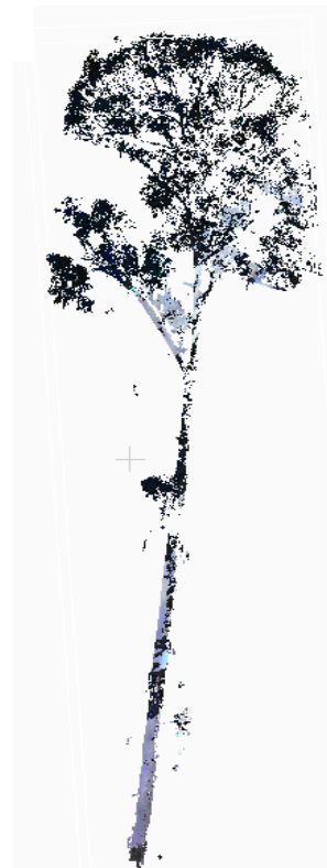
Figure 2. Examples of point cloud data. Combined point cloud of five scans looking laterally at the Eucalyptus Grove from the North (a). The same point cloud viewed from above (b). A single E. globulus tree that was extracted manually from the larger point cloud (c). With an estimated height of about 60m the tree in (c) is possibly the tallest Eucalyptus tree in North America. All three figures were generated in CloudCompare.
