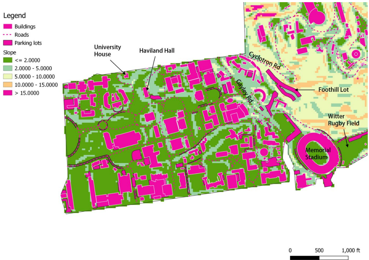
Figure 8. Map of the UCB campus showing slope and impervious surfaces. Green areas indicate low runoff generation and magenta areas indicate high runoff generation.
