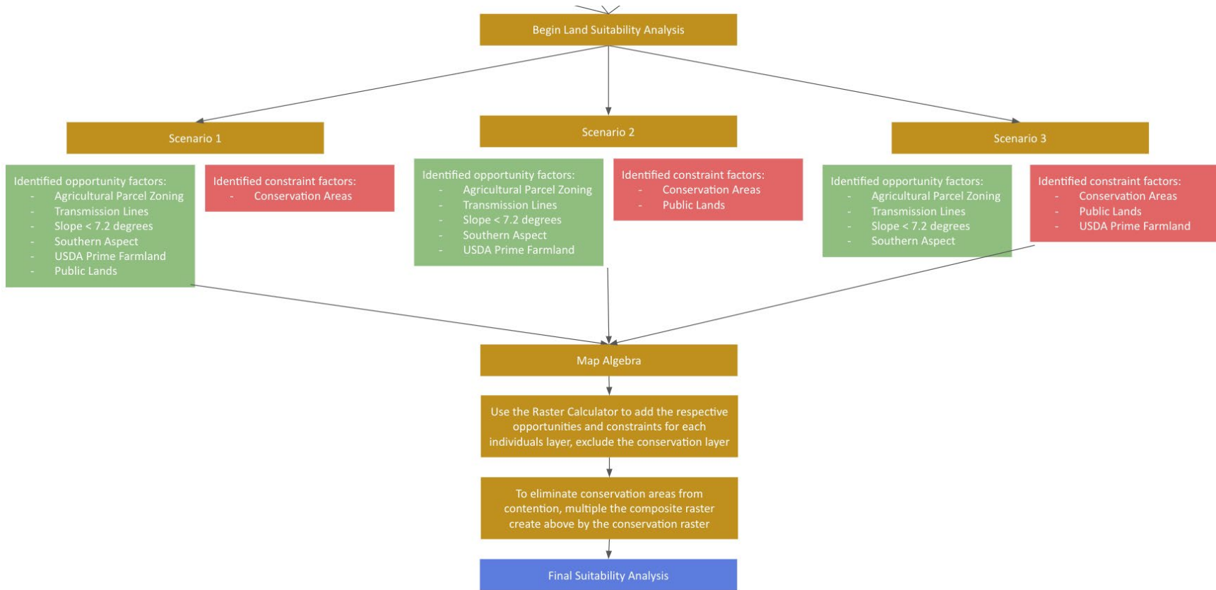
Figure A1: Land Suitability Analysis Flowchart. This figure shows the flow of logic as well as the ArcGIS functions used to execute each step in the Land Suitability Analysis.
