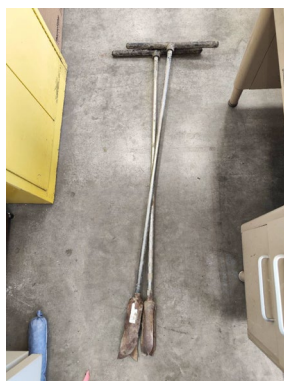
Figure 11. Auger digger used for soil sampling.
