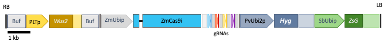
Figure 3: SbHT1 editing construct. The maize phospholipid transfer protein promoter drives Wus2 . The maize polyubiquitin promoter drives the intronized Cas9 sequence. The switchgrass polyubiquitin promoter drives Hyg , the hygromycin resistance gene. The sorghum polyubiquitin promoter drives ZsG , the green fluorescent protein.
