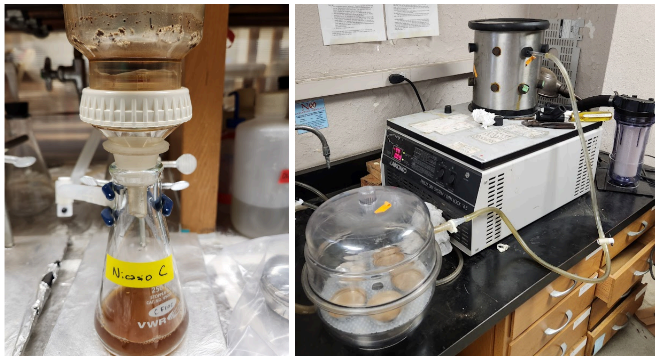
Fig 1. Laboratory techniques. (a) Hot Water Extraction of Nicasio sample C. Solution at the bottom of the vacuum filtering flask contains the labile carbon and the residue on the filter is the more persistent carbon. (b) Freeze dryer with HWE samples in the chamber. The freeze dryer allows for removal of water, leaving behind residue for later analysis, without applying heat.
