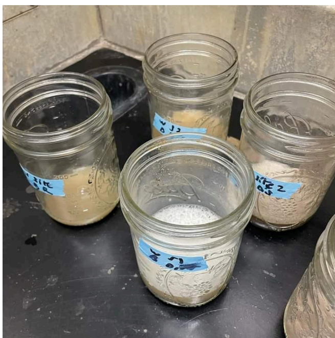
Figure 4. Removal of organic material in sediment samples through a 30% H_2O_2 digestion.
