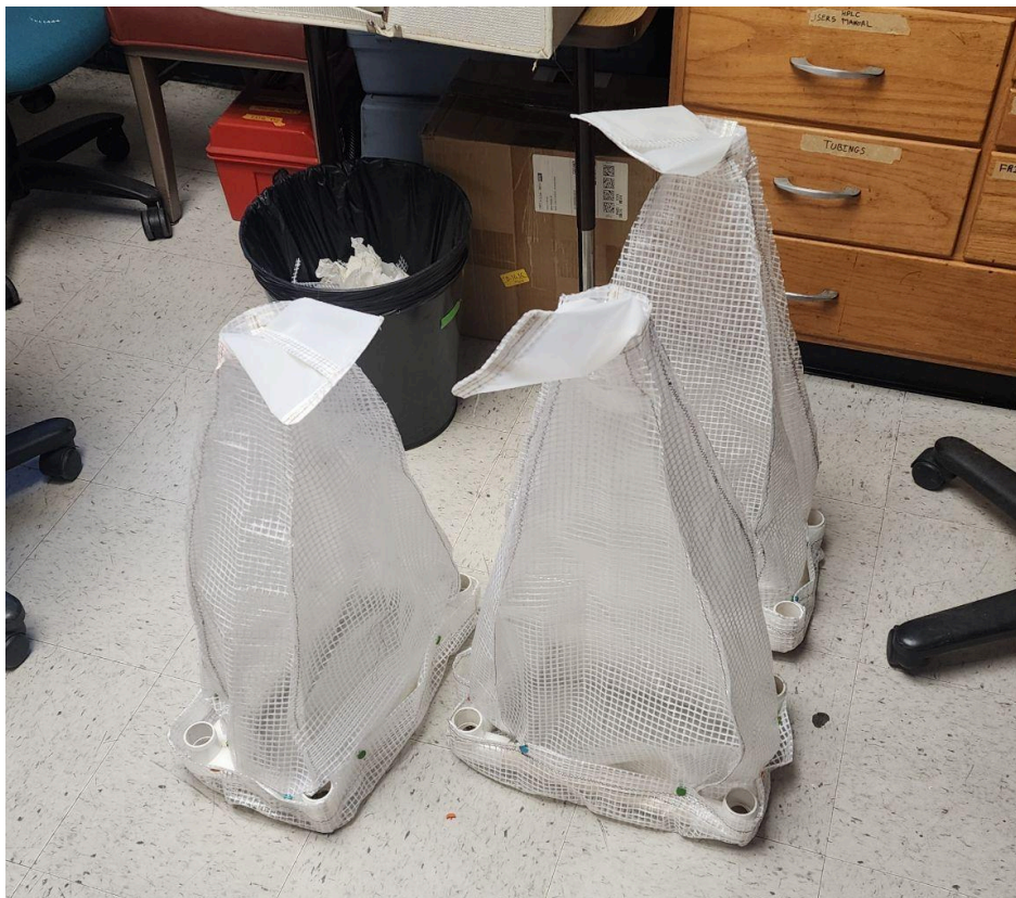
Figure 3. Completed drift nets.
