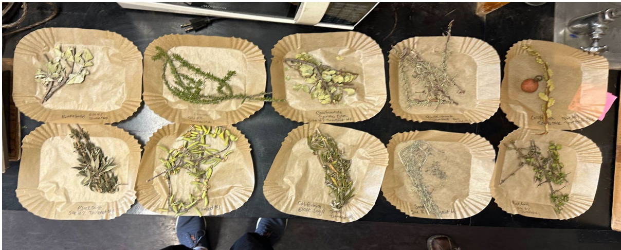
Figure 4. An image of assorted field clipping samples used to measure fuel moisture content that was recently removed from the drying oven.
