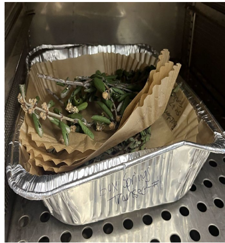
Figure 3. A picture of field clippings arranged on air fryer paper, and placed in aluminum tins within a drying oven.
