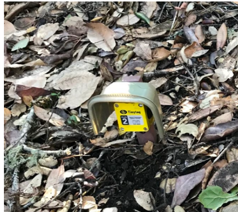
Figure 6. TinyTag Explorer logger set up at each sampling site. Credit: Will Lab, UC Berkeley ESPM
