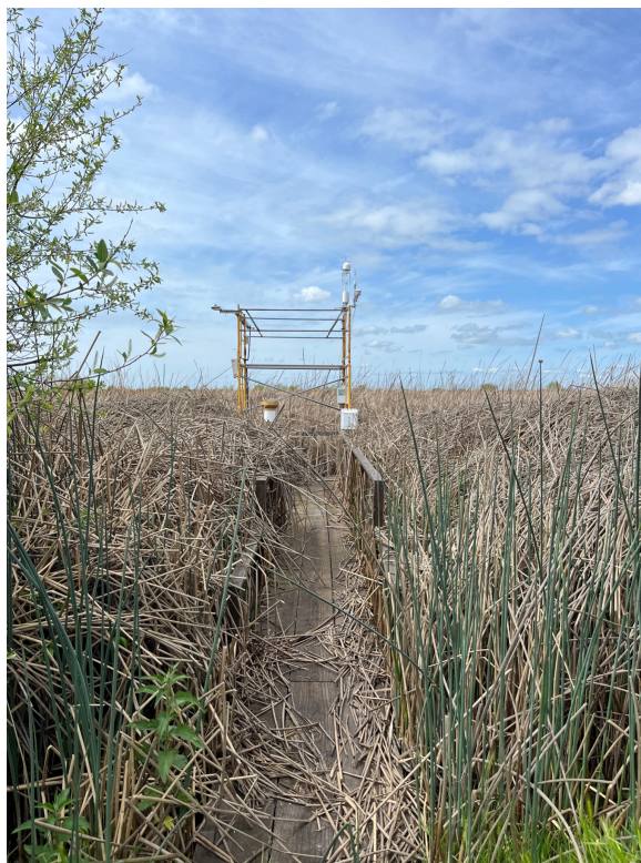
Figure 2. Eddy flux tower at the East End wetland site. This tower measures methane fluxes, carbon dioxide fluxes, Photosynthetically Active Radiation (PAR) air temperature, and GPP.
