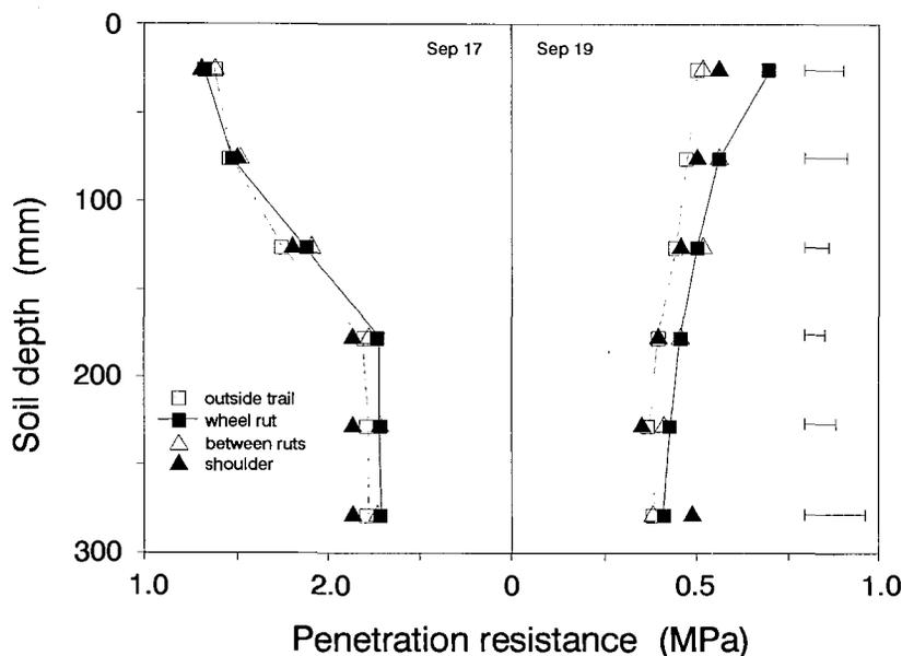
**Fig. 2. Penetration resistance at various positions across the historic Wadsworth Trail. Resistance as a function of depth was measured outside the trail, in the wheels ruts, between wheel ruts, and on the shoulder of the Trail before (17 September) and 24 h after (19 September) ponded infiltration. Error bars denote least significant difference ( $P = 0.10$ ).**
