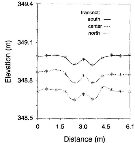
Fig. 1. Elevation (above mean sea level) along three transects of the historic Wadsworth Trail located near Morris, MN. Soil physical properties along each transect were measured at distances denoted by asterisks.
