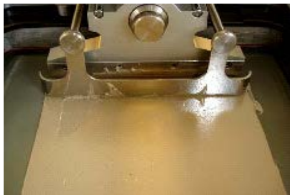
Figure 3: After conductive paste is dispensed onto the screen, the squeegee spreads it across the screen and presses it through onto the wafer.
