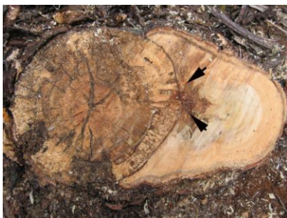
Figure 2. Pg135. E. globulus stump 24 months after harvest colonised by S. hirsutum . Arrows indicate where decay has entered from the stump into the coppice shoot.
