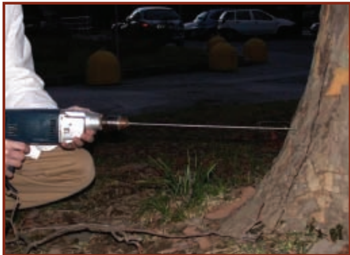
Figure 2. The double-fluted long drill bit used to collect sawdust from the base of standing trees.
