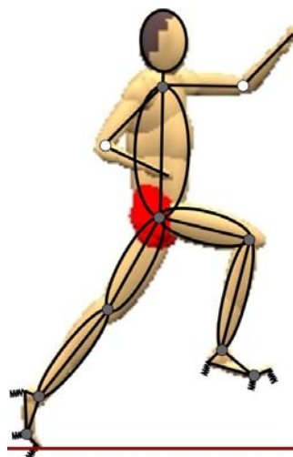
Figure 1. Thirteen-segment simulation model with wobbling masses within the shank, thigh, and trunk segments, torque drivers at the ball, ankle, knee, hip, and shoulder joints (grey circles), angle drivers at the elbow joints (white circles), and spring-dampers at three points on each foot.
