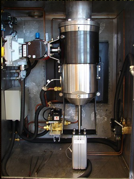
Neutron Activation analysis sample loading station.
