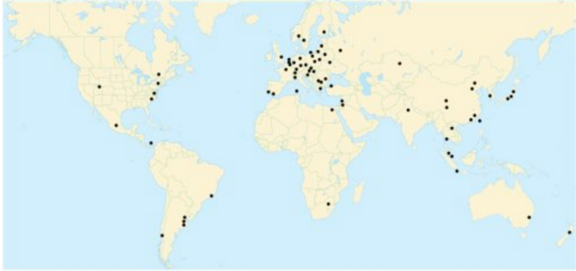
Figure 8. The atomic component of UTC is Temps Atomique International (TAI), which is based on atomic resonance measurements from some 200 contributors at locations, as shown above, around the world. The International Bureau of Weights and Measures (BIPM), located near Paris, maintains TAI with data received from these sites. Leap seconds are periodically introduced to adjust atomic time to keep it to within 0.9 seconds of Universal Time, adjusted for polar motion. The timing of their introduction is recommended by the International Earth Rotation and Reference Systems Service. The International Telecommunication Union, which defines the UTC broadcast recommendations, in 2012 will consider eliminating leap seconds from its definition. (Measurement device locations from BIPM website: http://www.bipm.org/en/scientific/tai/tai.html )
