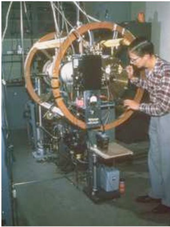
Figure 4. The U.S. National Institute of Standards and Technology (NIST) achieved the first accurate measurement of the frequency of cesium resonance in 1952. It used the instrument NBS-1, pictured above. At right is NIST-F1, the United States' present-day civilian time and frequency standard. It is believed to be accurate in measuring SI seconds at an error rate of only one second every 100 million years. (Photographs courtesy of NIST. Image at right by Geoffrey Wheeler.)
