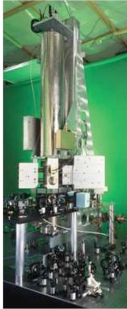
Figure 4. The U.S. National Institute of Standards and Technology (NIST) achieved the first accurate measurement of the frequency of cesium resonance in 1952. It used the instrument NBS-1, pictured above. At right is NIST-F1, the United States' present-day civilian time and frequency standard. It is believed to be accurate in measuring SI seconds at an error rate of only one second every 100 million years. (Photographs courtesy of NIST. Image at right by Geoffrey Wheeler.)
