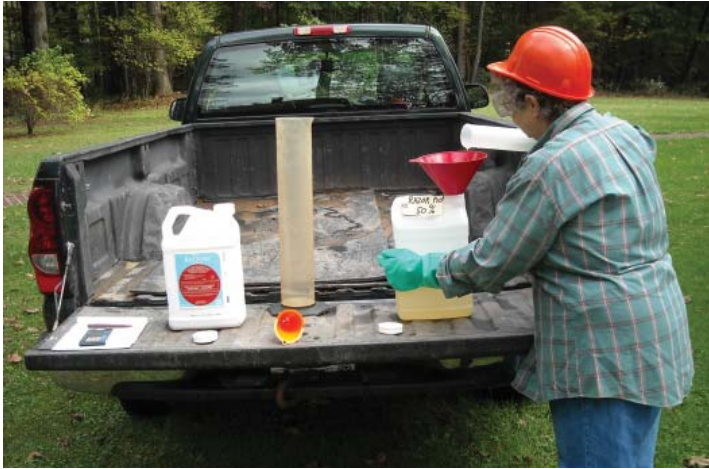
Figure 1.—Mixing herbicide solutions for a crop tree release operation. This worker is wearing personal protective equipment listed on the herbicide label. Other useful tools include a pocket calculator, graduated cylinder, and funnel.
