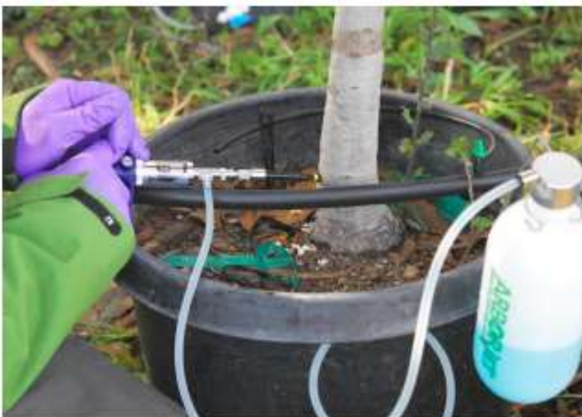
Injectons using 40 mL and 35 PSI (Moderate Pressure)
