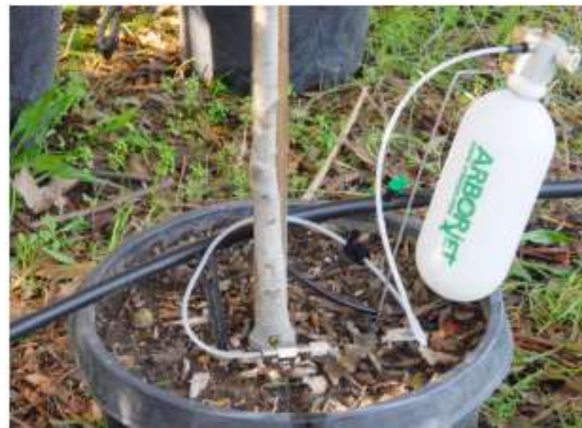
Injectons using 40 mL and 35 PSI (Moderate Pressure)
