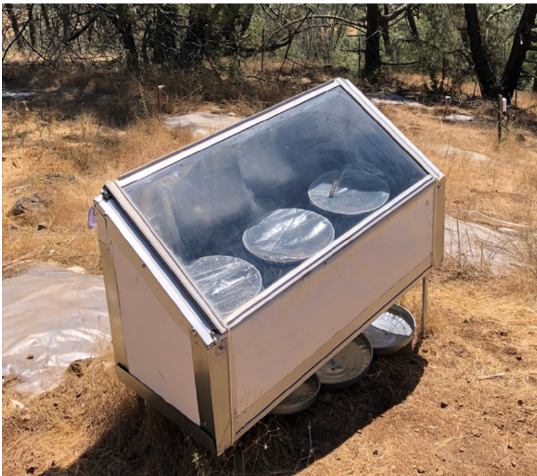
Insulated solar ovens bake soil to eliminate Phytophthora without sterilizing beneficial microorganisms. Courtesy photo by Janell Hillman, Santa Clara Valley Water District, used with permission.
