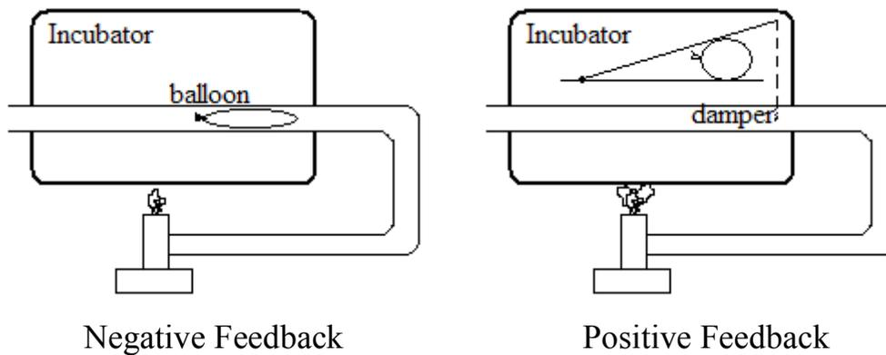
A thermostat affords one very simple case of feedback in everyday use. When the temperature in a room rises too high, the extra heat activates a switch which cuts off the source of heat, which in turn reduces the temperature. Illustrated above is a simplified mechanical model of a thermostat with negative feedback. As the incubator warms up,
