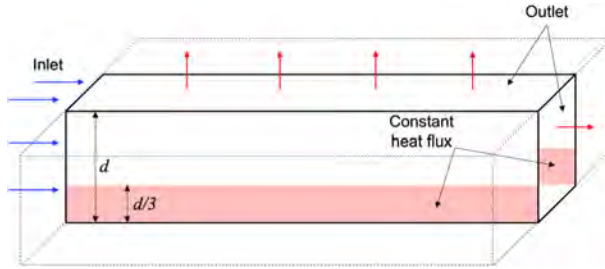
Figure 6. Computational domain corresponding to the spacing between the dowels.
