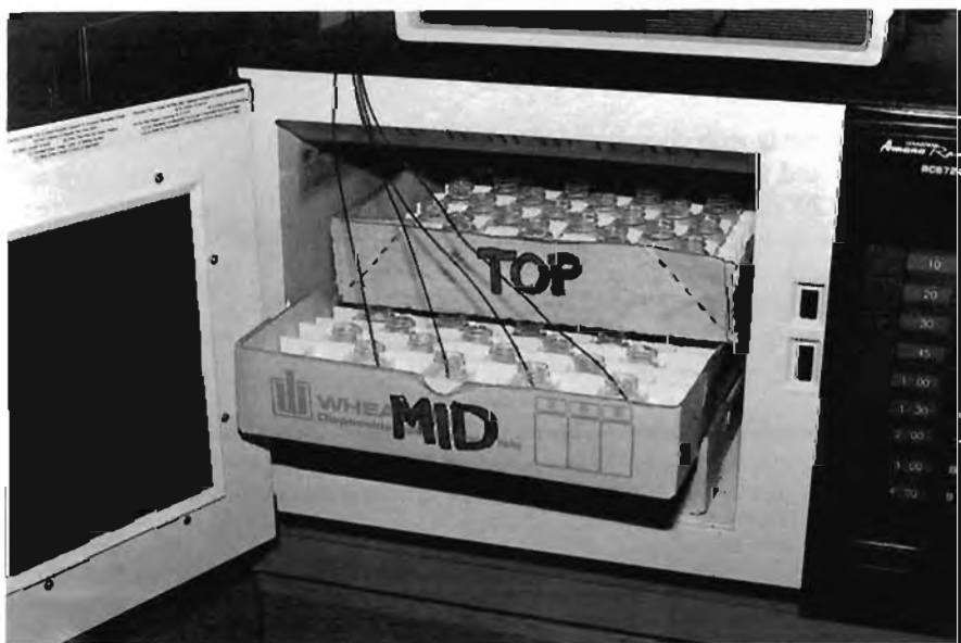
Figure 2. — Two vertically stacked cardboard trays containing 64 25-mL water-filled vials. Ovens producing 500-W, 1,000-W, and 2,000-W were run at full power for 4 minutes, 2 minutes, and 45 seconds, respectively. Initial and final temperature was recorded for each vial to calculate oven wattage.
