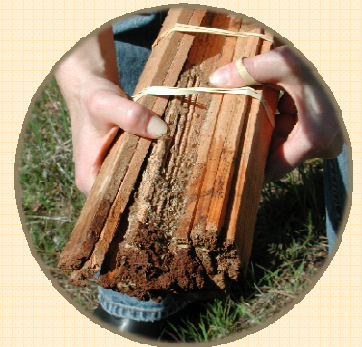
Wood bundle infested with subterranean termites
