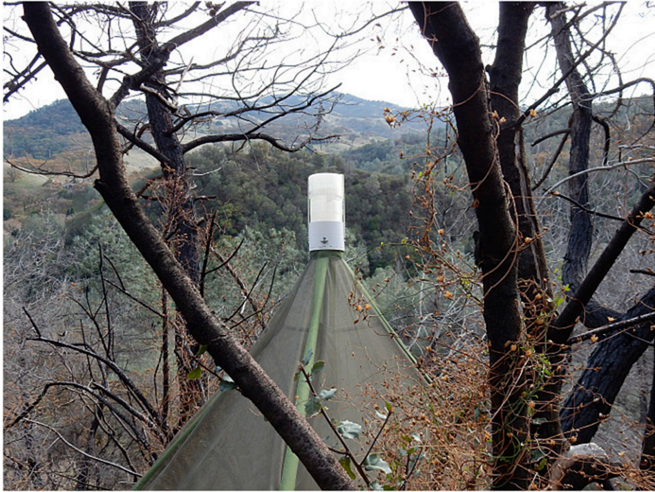
Figure 1. Trap with 3D printed trap head deployed at the Mt. Diablo site.
