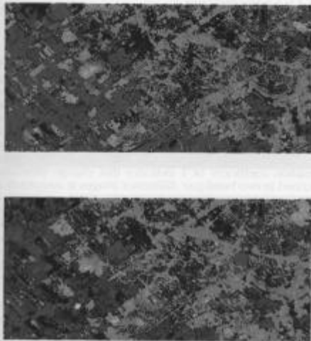
Figure 3. The 1985 (top) and 1986 (bottom) Landsat TM images of Kitchener/Waterloo, Ontario. Both images are black-and-white versions of colour displays by assigning TM bands 2, 3, and 4 with blue, green, and red colour guns, respectively.
